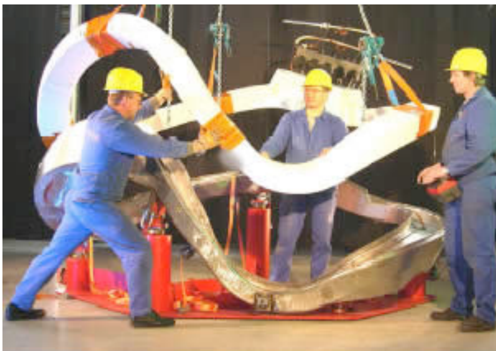
Wendelstein 7-X Stellarator magnets are complex
