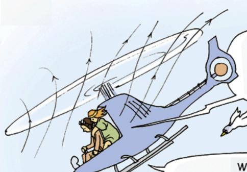
OK, now the air flow is inverted. It's going from the top to the bottom. My helicopter has been turned into an autogyro. The motor part, the rotor's autorotation, pulls the rest.
