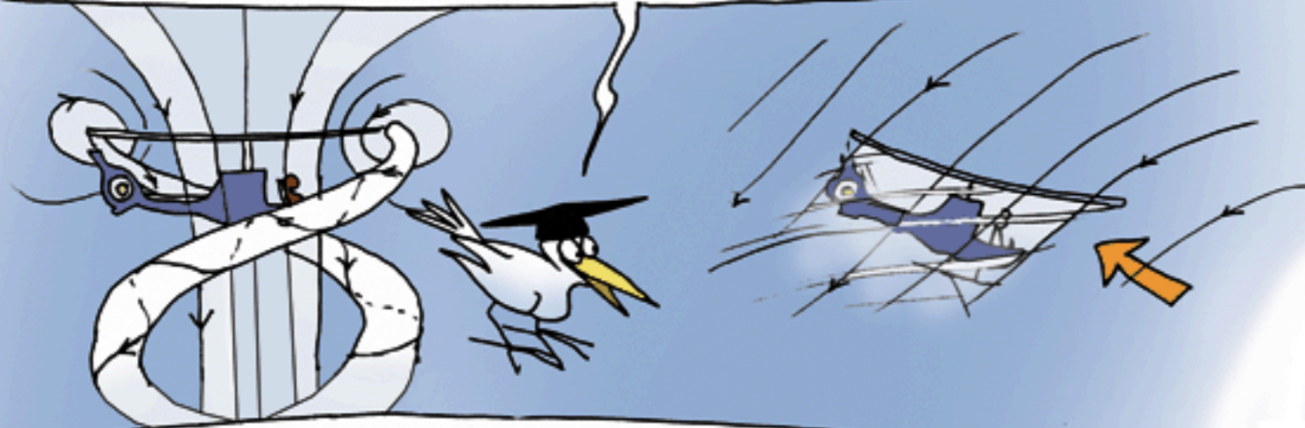
Less loss due to blade tip vortices
