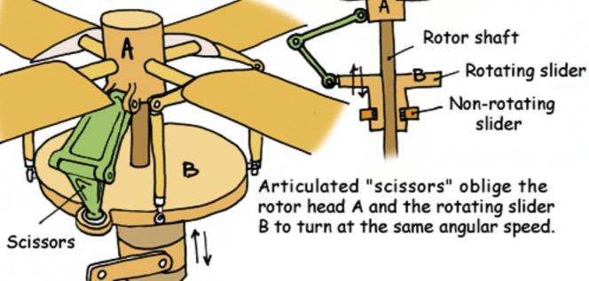
With such a system we can vary all the blades of a rotor at the same time by acting on the non rotating slider, linked via a ball-bearing and a rotating slider A, which retransmits the order to the blades via levers.
