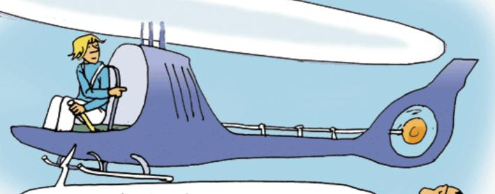
So I adapted the same system to the tail rotor, antitorque, so as to avoid changes of direction when I changed the general pitch, and I added a foot control, a pedal, that lets me hover.
