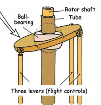
To make something work straight that is off kilter, the solution is a **BALL-BEARING**
