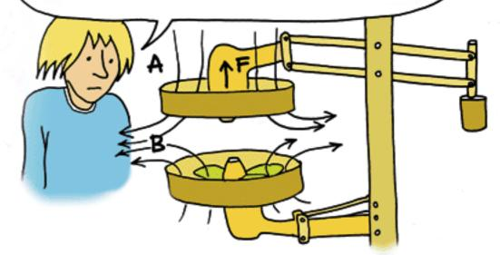
At equal power, the force of ascension exerted on the fan A is greater when it is running facing fan B, which pushes air in the opposite direction, than if fan A was runing alone.
