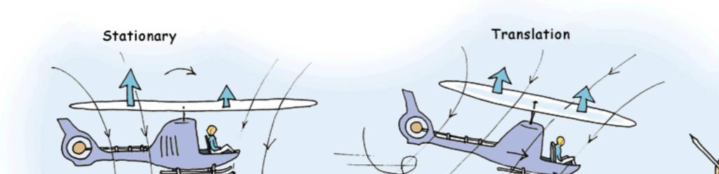
If I could increase the lift of the rotor's blades when these are towards the back and increase it when they are towards the front, using CYCLIC PITCH VARIATION, that would make the machine tilt and start a TRANSLATION movement.
