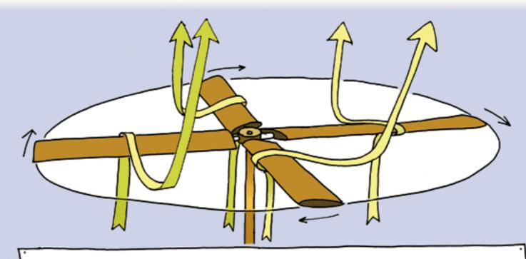
Here the flow is reattached to the blade's edge
