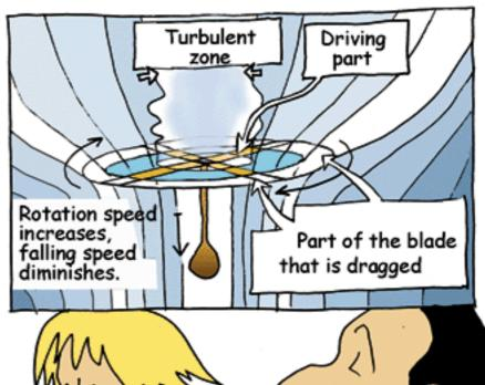
The rotation speed stabilises when the two couples balance each other. Then the autorotation regime is completely established and the speed of descent is minimal.
