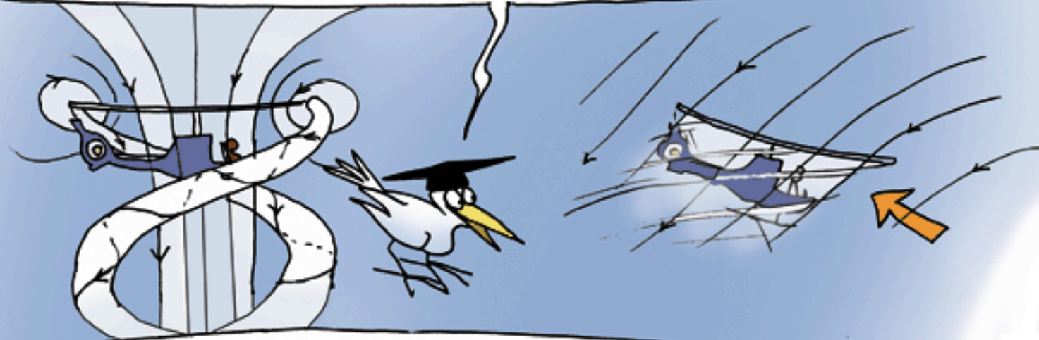
Less loss due to blade tip vortices
