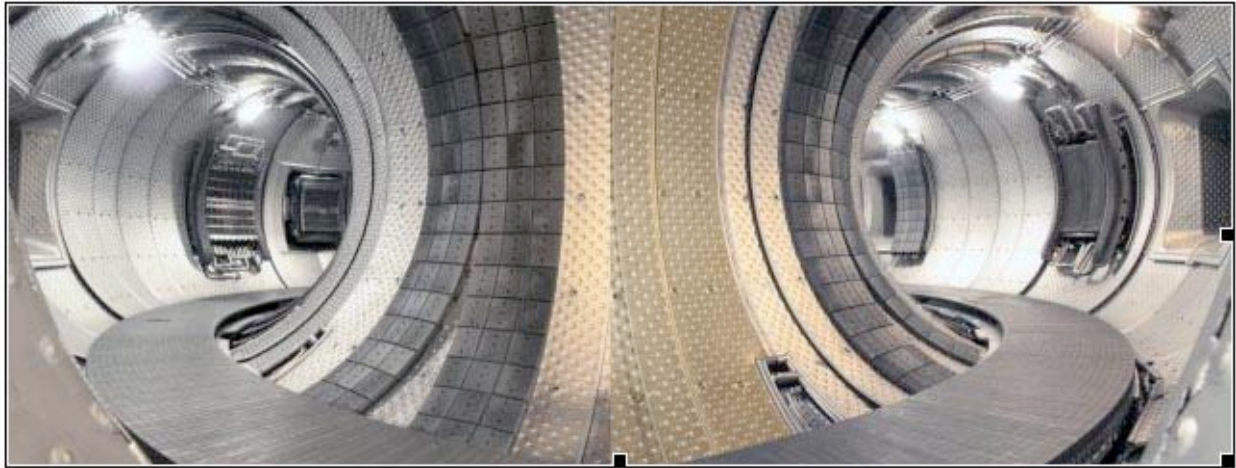
The Tore Supra limiter covered with carbon plates
