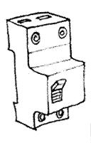
To be complete, we'll finish by mentioning the DIFFERENTIAL CIRCUIT BREAKER. This is an electromagnetic apparatus that controls the absolute values that pass through the live and neutral when an installation is being supplied with electricity. If the apparatus detects a difference of 10 to 20 milliamperes, it means that there is a current leak somewhere so the circuit-breaker automatically cuts the current off
